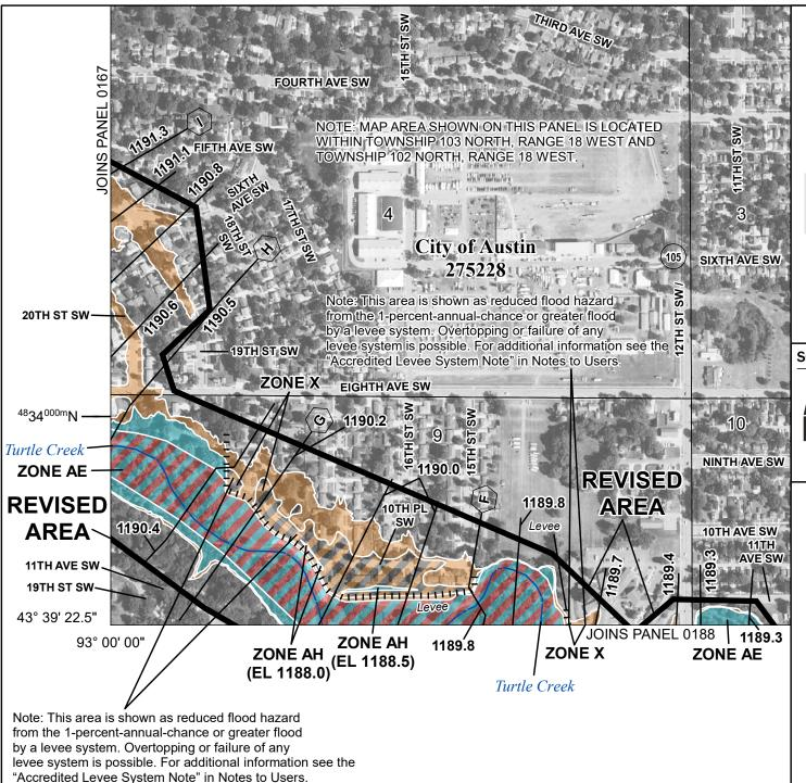
Without Base Flood Elevation (BFE) With BFE or Depth Zone AE, AO, AH, VE, AR SPECIAL FLOOD Regulatory Floodway HAZARD AREAS 0.2% Annual Chance Flood Hazard, Areas of 1% annual chance flood with average depth less than one foot or with drainage areas of less than one square mile Zone X **Future Conditions 1% Annual**
