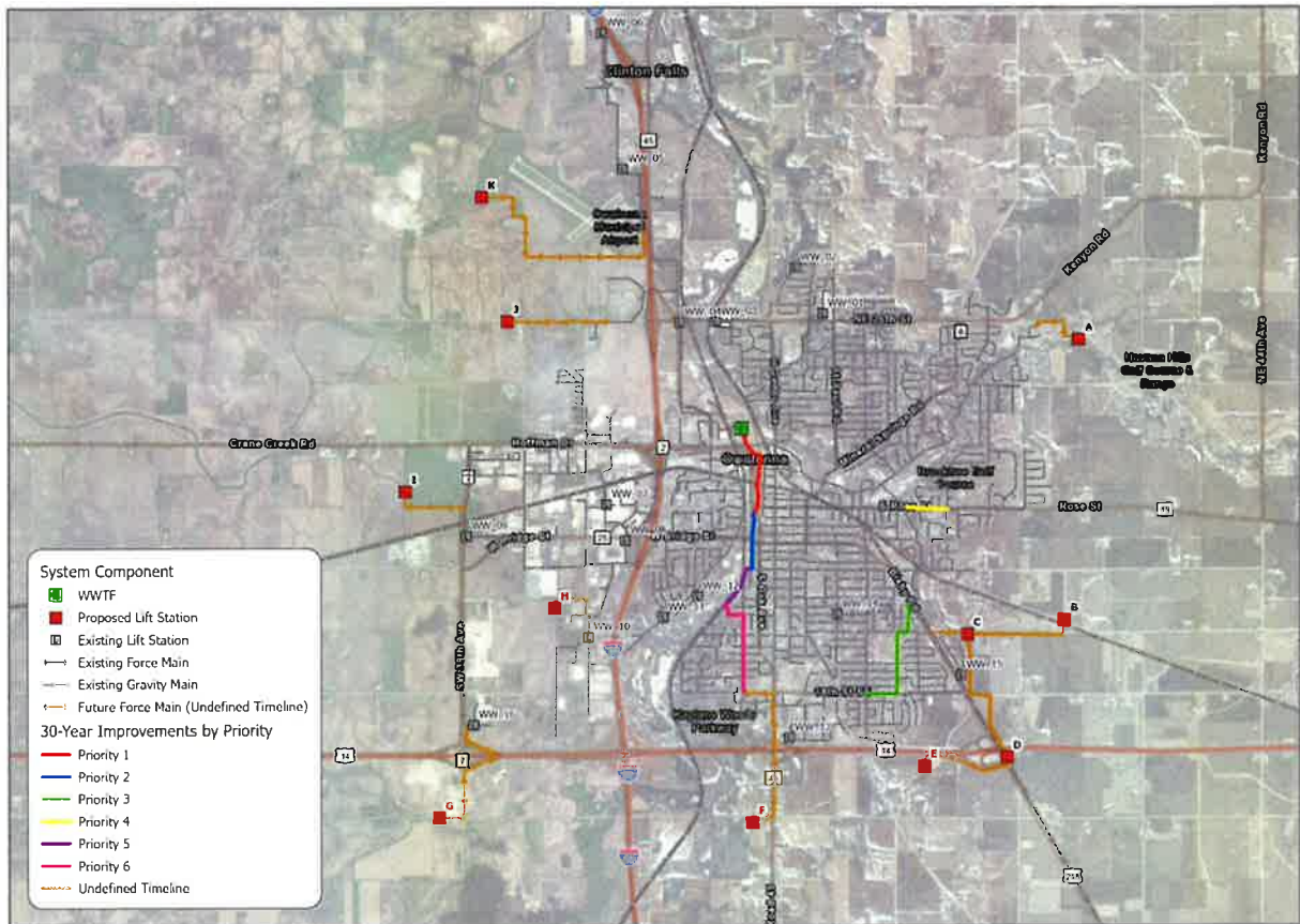
Figure 6.3 Wastewater 30-Year Improvements Prioritization
